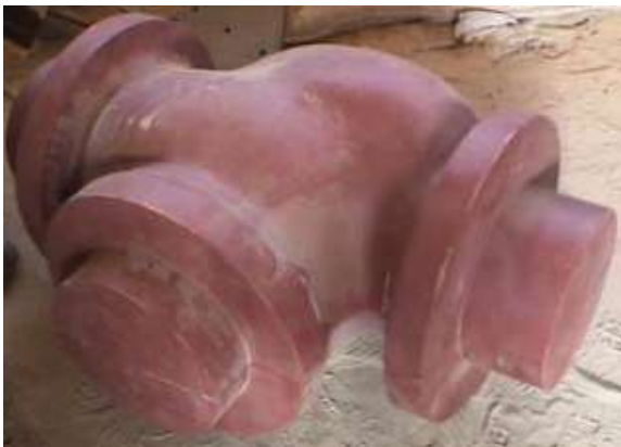
SUCTION VALVE -P1021 & 1022 P/F MASONIELAN CONTROL VALVE MODEL NO : 38-41911 TYPE: GLOBE SINGLE SEAT CV :1400 SIZE: 12
