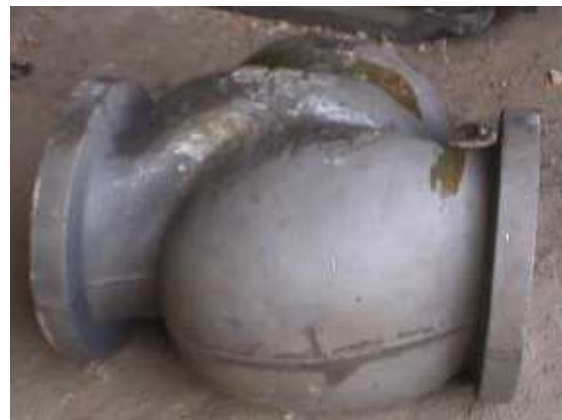
SUCTION VALVE -P1021 & 1022 P/F MASONIELAN CONTROL VALVE MODEL NO : 38-41911 TYPE: GLOBE SINGLE SEAT CV :1400 SIZE: 12
